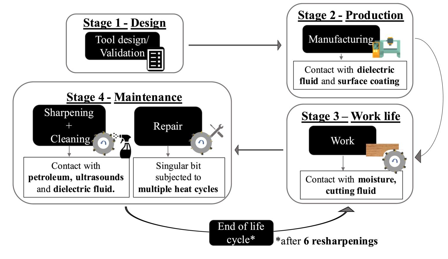
Figure 1 – Typical life cycle of a milling tool [2].
